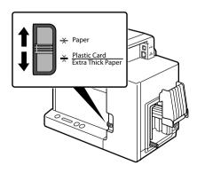
Set the lever to the appropriate position according to the paper to be printed on.
