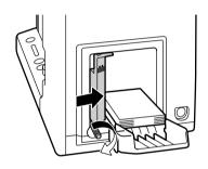
4. Adjust the side guides to the paper edge, and secure them in place with the screw.
