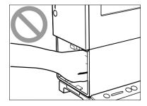
When the feeder lift tray is moving, do not touch it. Also, do not insert your hand or place objects below the tray. Doing so can cause injury or malfunction.
