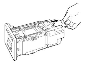
• Check that the paper is not jammed further in the transport unit. If paper is jammed, remove it.
